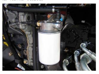
Lube Point(s) - Replaceable Element Interval - Every year or 600 hours of operation
