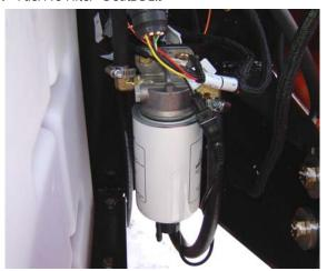
Lube Point(s) - Replaceable Element Interval - Drain water daily; Every year or 600 hours of operation
