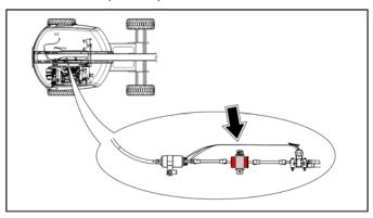
Lube Point(s) - Replaceable Element Interval - Every 6 months or 300 hours of operation
