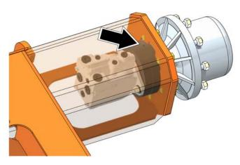
Lube Point(s) - Fill Plug Capacity - 2.7 oz. (89 mL) Lube - DTE-10 Excel 32 Interval - Change as necessary
