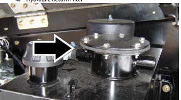
Interval - Change after first 50 hours and every 6 months or 300 hours thereafter or whenever Charge Filter is replaced
