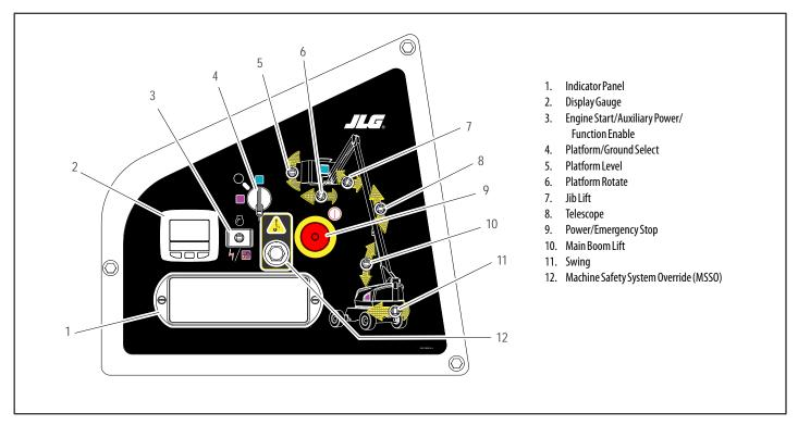
Figure 3-4. Ground Control Console - 460SJ w/MSSO (CE Only)
