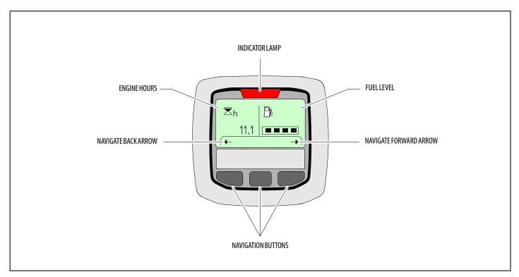
Figure 3-10. Ground Control Console Display Gauge
