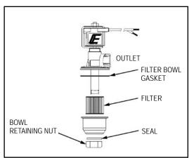
Figure 6-13. Kubota Filter Lock Assembly
