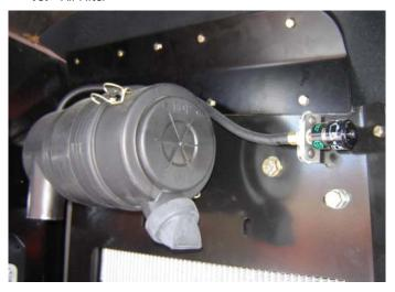
Lube Point(s) - Replaceable Element Interval - Every 6 months or 300 hours of operation or as indicated by the condition indicator Comments - Check Dust Valve daily
