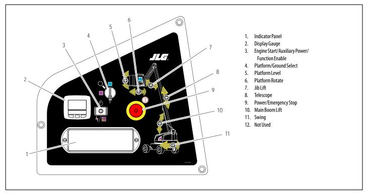
Figure 3-3. Ground Control Console - 460SJ
