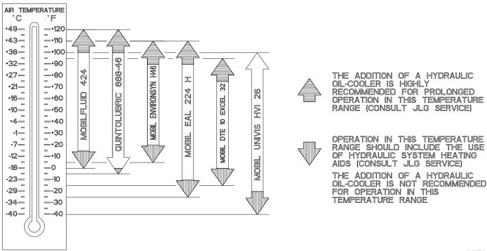
Figure 6-2. Hydraulic Oil Operation Chart - Sheet 1 of 2
