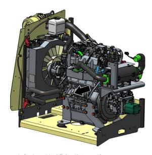
Lube Point(s) - Fill Cap/Spin-on Element Capacity - 2.5 gal. (9.5 L) w/filter
