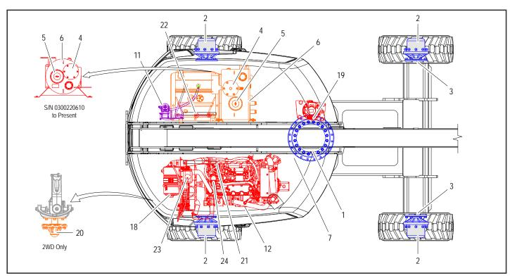
Figure 6-11. Operator Maintenance and Lubrication Diagram - Kubota Engine
