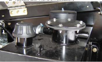
Lube Point(s) - Fill Cap Capacity - 32.5 gal tank (123 L) 40.0 gal system (151 L) Lube - HO Interval - Check Level daily; Change every 2 years or 1200 hours of operation
