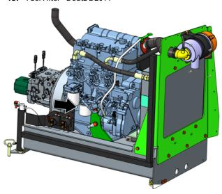
Lube Point(s) - Replaceable Element Interval - Every year or 500 hours of operation
