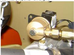
Interval - 3 Months or 150 hours of operation Comments - Replace filter. Refer to Section 6.5, Propane Fuel Filter Replacement (GM Engine)
