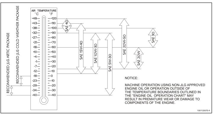
Figure 6-7. Engine Oil Operation Chart - Kubota
