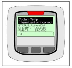
Figure 3-9. Engine Diagnostic Screen
