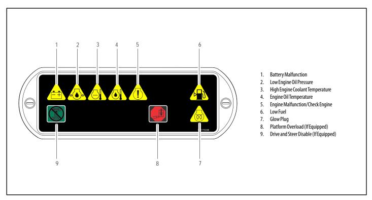
Figure 3-5. Ground Control Indicator Panel
