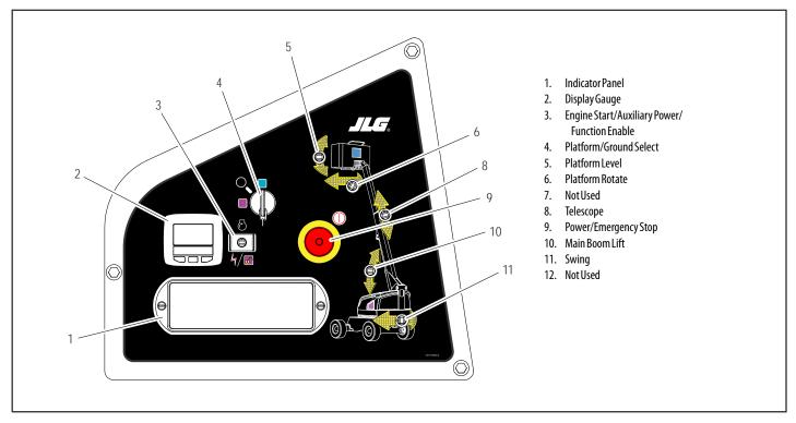
Figure 3-1. Ground Control Console - 400S
