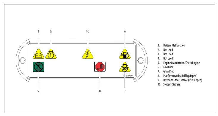
Figure 3-6. Ground Control Indicator Panel - Kubota Engine
