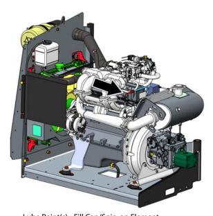
Lube Point(s) - Fill Cap/Spin-on Element
