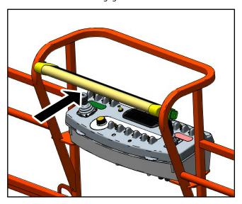
**NOTE:** If equipped, ensure the Skyguard beacon illuminates when Sky-Guard is activated.
