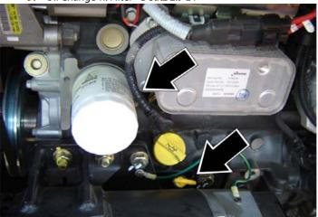
Lube Point(s) - Fill Cap/Spin-on Element
