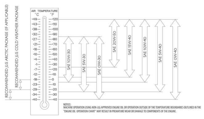
Figure 6-4. Engine Operating Temperature Specifications - Deutz
