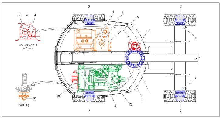
Figure 6-9. Operator Maintenance and Lubrication Diagram - Deutz 2011L Engine
