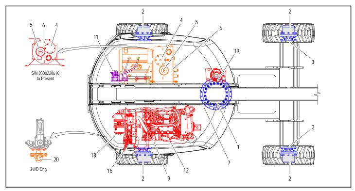
Figure 6-8. Operator Maintenance and Lubrication Diagram - Deutz 2.9L Engine
