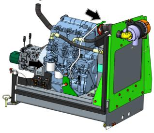
Lube Point(s) - Fill Cap/Spin-on Element Capacity - 10 Quarts (9.5 L) w/Filter
