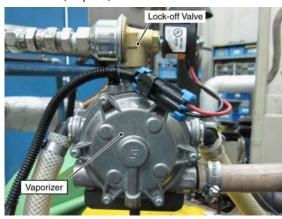
Interval - Every year or 1000 hours of operation Comments - Replace filter. Refer to Section 6.6, Propane Fuel Filter Replacement (Kubota Engine)
