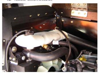
Lube Point(s) - Fill Cap Capacity - 2.9 Gallon (11.3 L) Lube - Anti-Freeze Interval - Check level daily; change every 1000 hours or 2 years, whichever comes first
