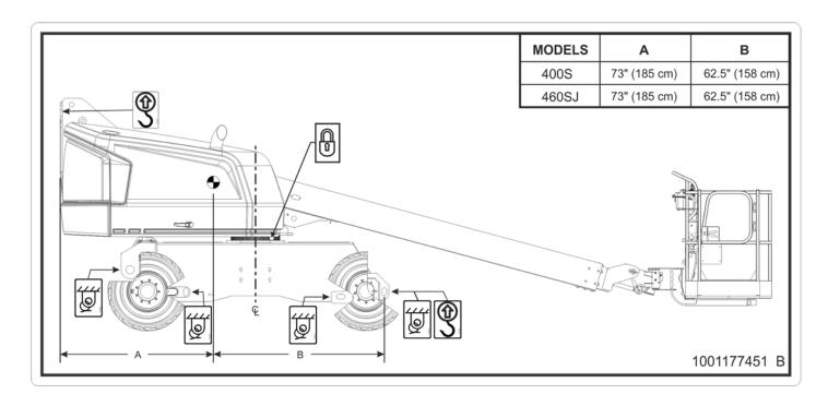
Figure 4-5. Lifting and Tie Down Chart
